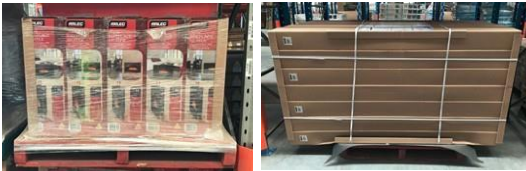
Examples of corner posts in use
